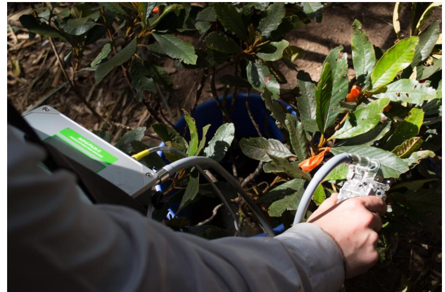
Chlorophyll fluorescence using a MINI-PAM-II fluorometer
