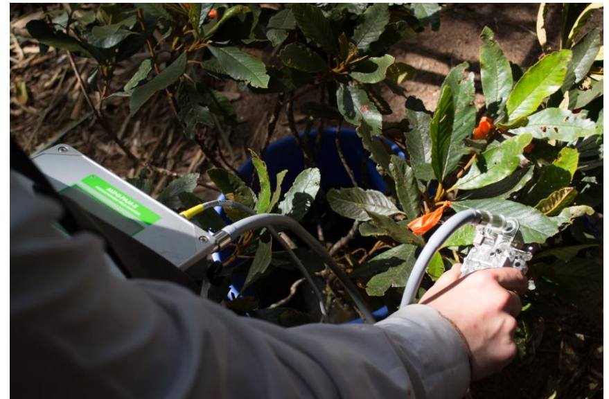
Chlorophyll fluorescence using a MINI-PAM-II fluorometer
